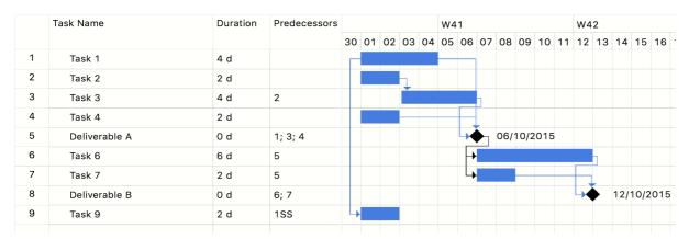
Then we perform the **backward pass**, to compute the latest dates. Starting from the end node, whose latest start and latest end are set to the earliest end, we set a task's latest end by taking the lowest latest end of all the successors. We then compute the latest start by subtracting a task's duration to its latest end.
