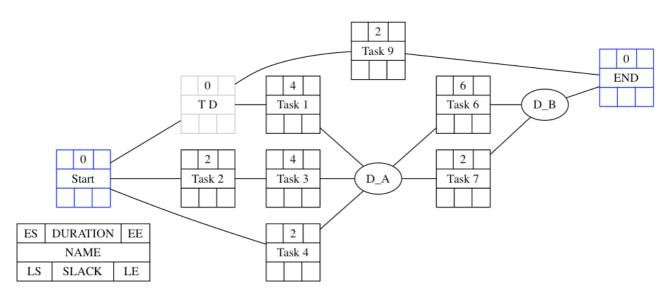
Notice that we have added the dummy node T\_D to manage the SS dependency between Task 1 and Task 9; for all tasks we have used a notation which allows us to record all relevant information of a task, namely Earliest Start, Duration, Earliest End, Latest Start, Slack, and Latest End; only for the sake of clarity, we have used a circle for the deliverables—we will have to change it in the next
